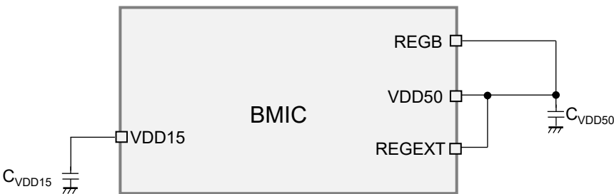
Fig. 3.3.2 VDD50 low power mode setting for REGEXT= 5V
