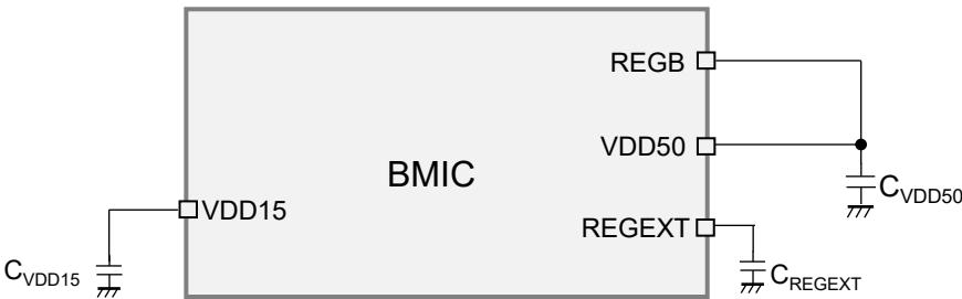
Fig. 3.3.1 VDD50 low power mode setting for REGEXT= 3.3V
