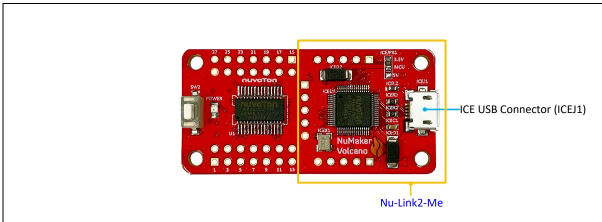
Figure 3-4 External Power Supply Sources on Nu-Link2-Me
