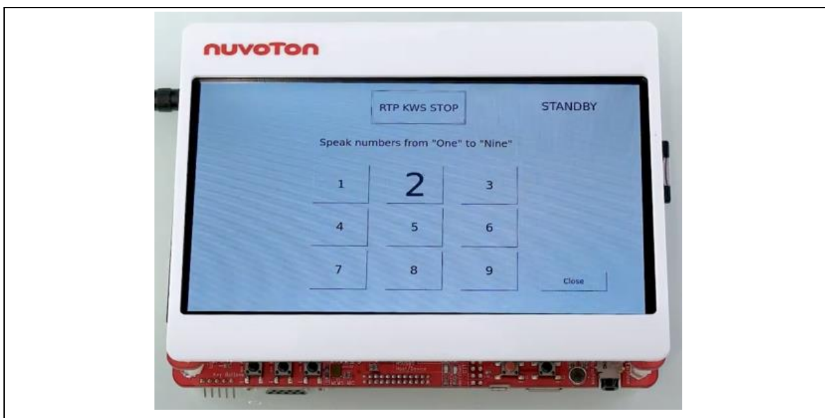
Figure 4-10 Keyword Spotting by RTP M4 Demonstration
