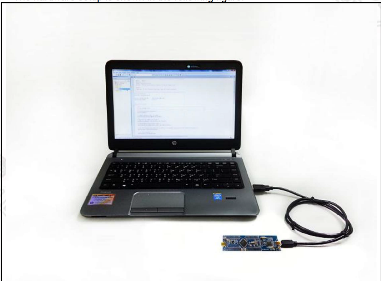
Figure 4-1 NuTiny- SDK-M453 Hardware Setup
