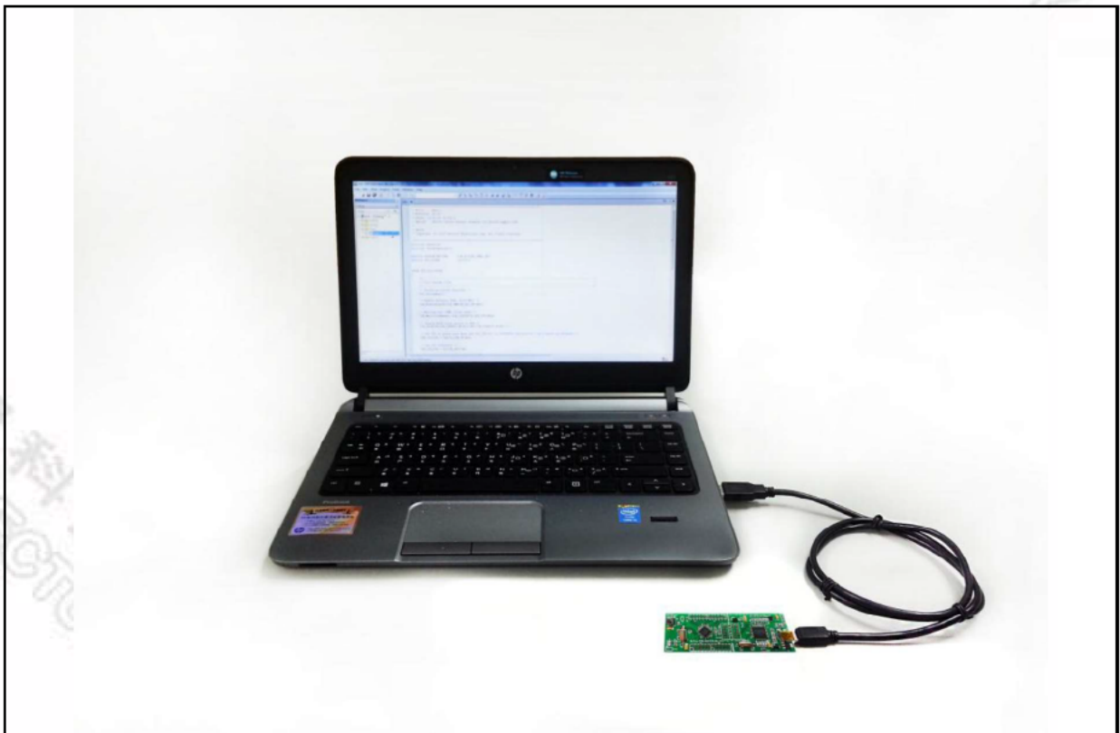
Figure 4-1 NuTiny-SDK-NUC029LAN Hardware Setup
