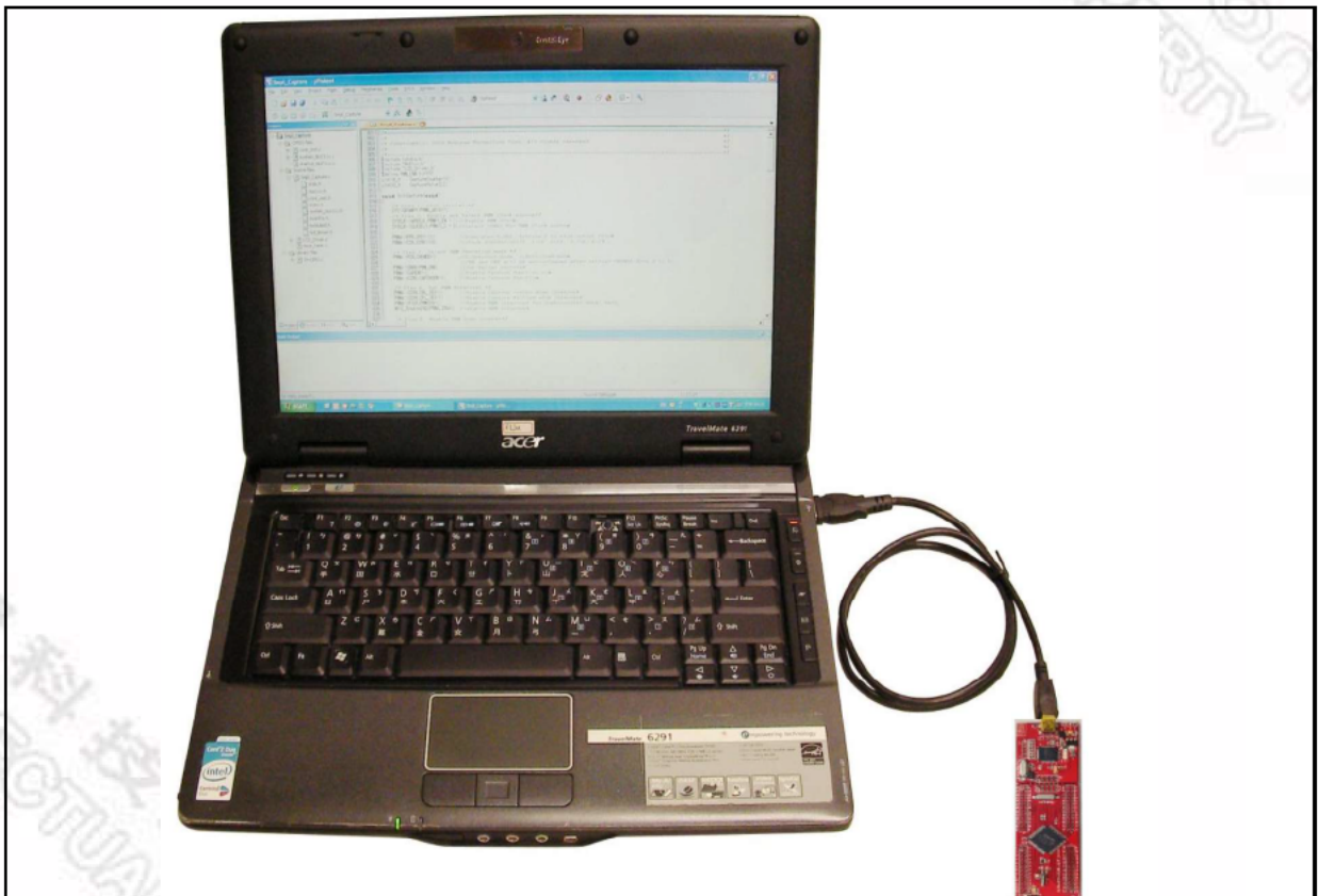
Figure 3-1 NuTiny-SDK-NUC200 Hardware Setup
