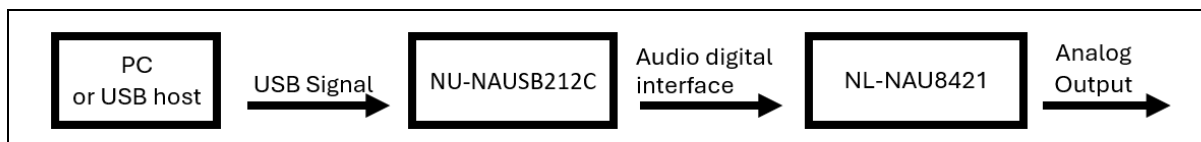
Figure 2-5 Signal Path of NU-NAUSB2I2C and NL-NAU8421
