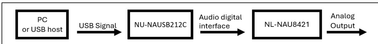
Figure 2-5 Signal Path of NU-NAUSB2I2C and NL-NAU8421
