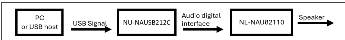
Figure 2-5 Signal Path of NU-NAUSB212C and NL-NAU82110
