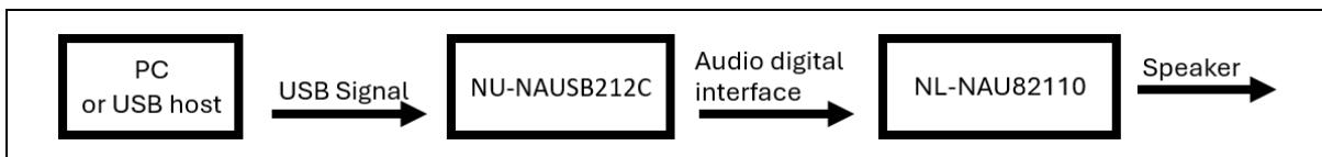
Figure 2-5 Signal Path of NU-NAUSB2I2C and NL-NAU82110
