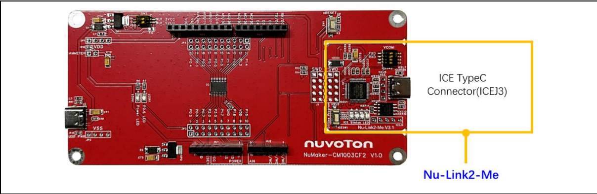
Figure 3-5 External Power Supply Sources on Nu-Link2-Me
