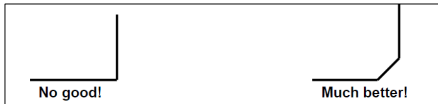
Figure 9.3.1 PCB layout trace notice for RMI signals
